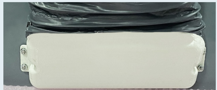
Simple modification on side panel to install duct for dispensing.
