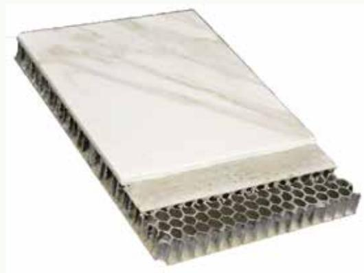
Breakdown showing honeycomb, fiberglass skin and 1/8-in. stone
