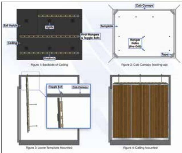
Breakout of island downlight ceiling; drawing courtesy of LWI Elevator Panel Co.
