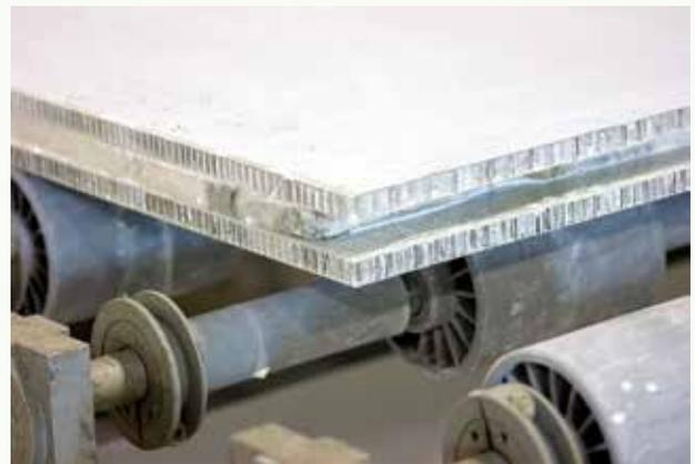
3/4-in. stone slab with honeycomb panel on both sides
