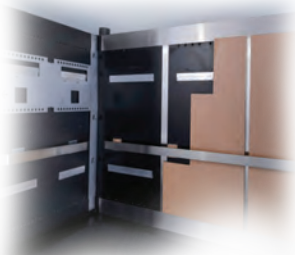
Complete cab interior packages Above photo shows install template on left and finished panels on right
