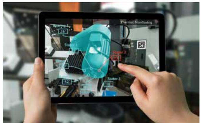
Real-time data displayed on an AR tablet can be used to optimize equipment performance and maintenance, detect and proactively correct causes for future failures, and train technicians.
